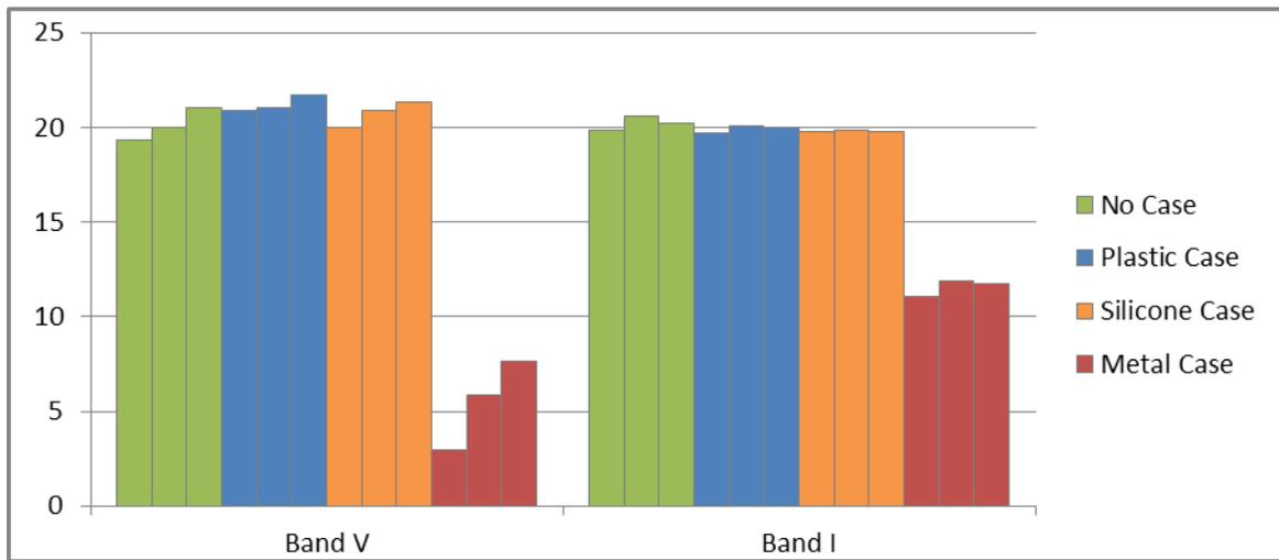
Figure 6, HSPA -TRP for Phone A, band I and V when using different covers. The bars are from lowest to highest frequency channel.
