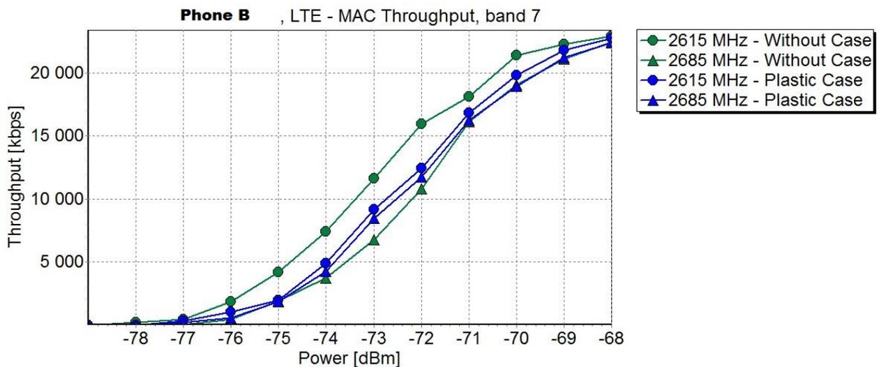
Figure 9, LTE - MAC Throughput for Phone B band 7
