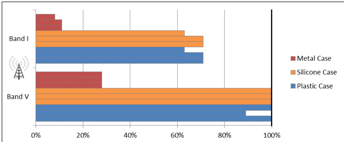
Figure 7, Relative distance from base station for different covers in order to get the same throughput. 100 percent represent the distance needed without a cover.
