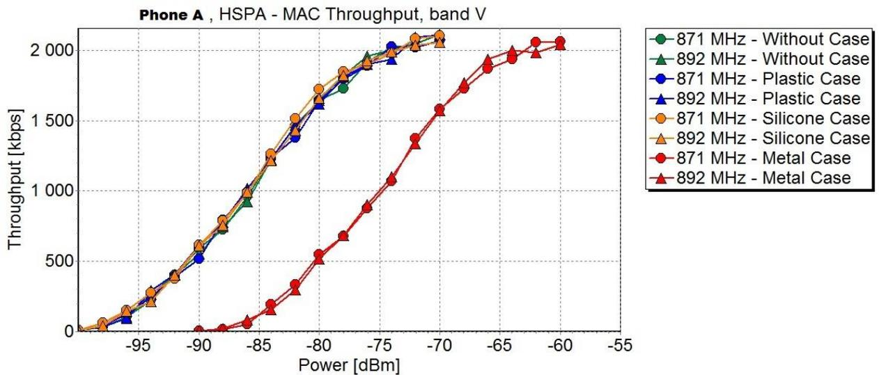
Figure 5, HSPA – MAC Throughput for Phone A, band V
