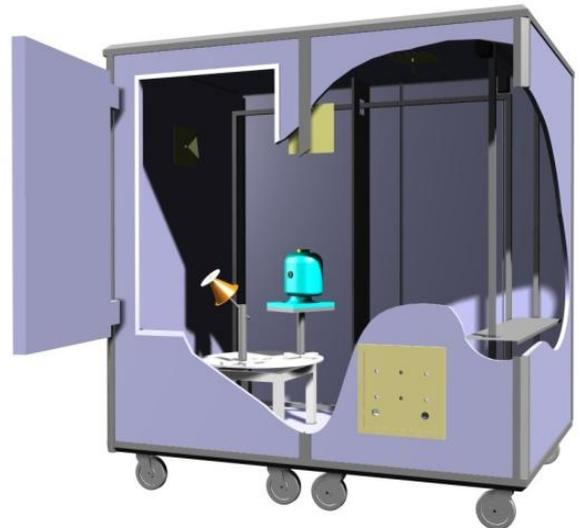
Figure 1. Drawing of the Bluetest HP700 reverberation chamber
