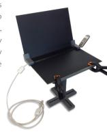
The Laptop Ground Plane Phantom is used for measurements on USB devices. It is designed according to the specification in 3GPP TS 34.114 and comes with a 1 m USB cable and two clamps for easy and flexible attachment to the Small Table.
