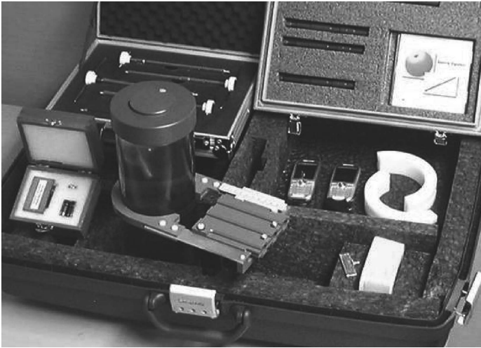
Figure 12.5 Test kit used in the round-robin campaign, together with suitcase used for shipping.
